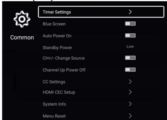
**Channel +/- Change Source:** If enabled, once the TV reaches the top or the bottom of its channel map, it will channel to other enabled sources.
