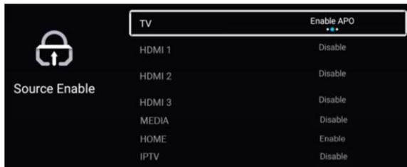
**Source Enable:** This menu is where you will enable/disable the TV's sources/inputs. Each source can be set to Disable, Enable/APO (auto-power-on), Enable/NAPO (no-auto-power-on). At least one of TV, HDMI1, HDMI2, HDMI3 must be enabled.
