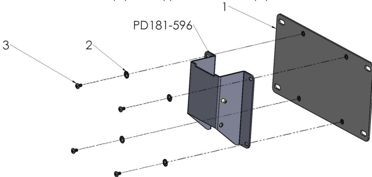
2. Secure the **PD181-677** adapter plate (#1) to the PDi TV (not included) using four (4) **PDIPPHMSM5X810** screws for a PDi 29" TV or four (4) **PDIPPHMSM6X110** (#5) screws for a PDi 32" plastic TV or four (4) **PDIPPHMSM6X18** screws (#6) for a **PDI-A32** TV, as shown.
