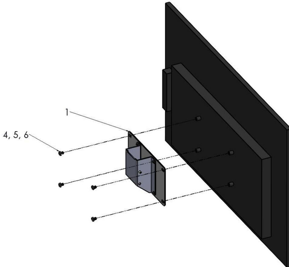
3. Connect the **PD181-596** wall bracket (not included) to the **PD181-697** wall bracket (not included) (both parts from PD168-103 mount) using the two (2) **PDIPPBHSCS103250** screws and two (2) **PDIITLW10** washers. Ensure the pivot bolts are retained in the "L" shaped slot as shown.
