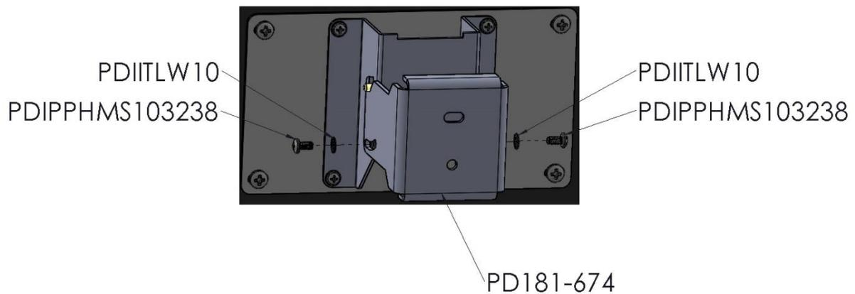
4. The TV's tilt can be adjusted by loosening both Pilfer Screws, adjusting tilting, and then tightening the (2) **PDIPPBHSCS103250** pilfer proof head socket screws.
