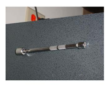
4. LOCATE PDI-519 ADJUSTMENT TOOL ON THE HEX BOLT IN THE REAR OF THE ARM, TURN BOLT 9 FULL TURNS COUNTERCLOCKWISE
