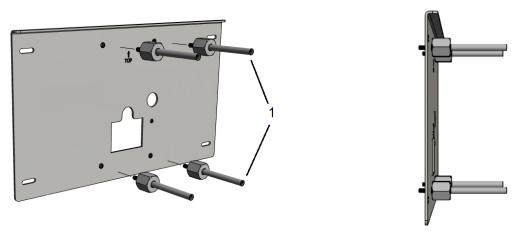
2. Install PDI-179C parts (backer plate and extension) onto spacers in order shown with casting opening at the top.
