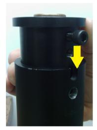
Step 4: Install (1) PDISHCS252088 Pilfer proof screw as shown.
