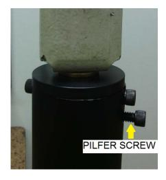
Step 5: Install arm and tighten all three new screws and original set screw. Confirm that arm will not pull out of bushing and rotates freely
