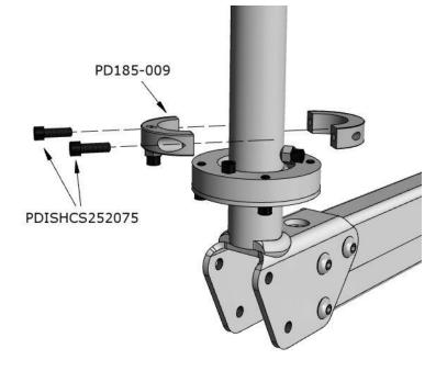
4. ROTATE CEILING MOUNT ARM TO VERIFY PROPER CONTACT OF THE NEW STOP BOLT AND EXISTING STOP BOLT IN THE PDI-589 STOP COLLAR.
