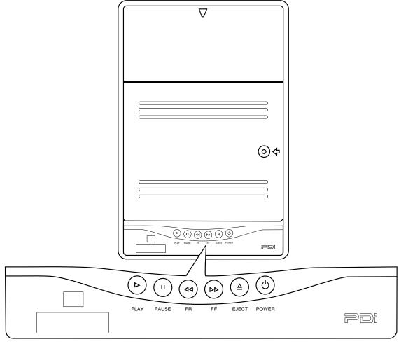
The front control buttons serve dual purposes: the first is control of the disc during normal movie Playback, and the second when the DVD Disk Menu is active.
