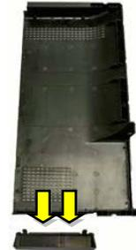
2. Attach the panel accessory that came with the computer module by inserting it in the slot where the other panel accessory was located.
