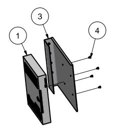
Connect the A/V and power cables to the DVD player, routing all of the cables up. Attach the DVD player (#1) to the PD181-668 bracket (#3) with four PDITPHMSM4X76 screws (#4).
