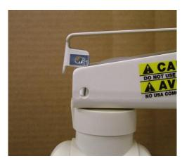
8. INSTALL SUPPLIED SCREWS IN FRONT OF NOSE TO HOLD NOSE COVER IN PLACE (IF ARM COVER KIT IS TO BE INSTALLED, FOLLOW INSTRUCTIONS FOR PIN STORAGE WHEN USED WITH COVER KIT).
