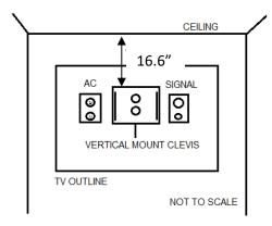
Attach the four (4) PD181-825 Adapter Brackets (#2) to the back of the TV using four (4) PDIPPHMSM6X110 screws (#1), leave screws finger tight.
