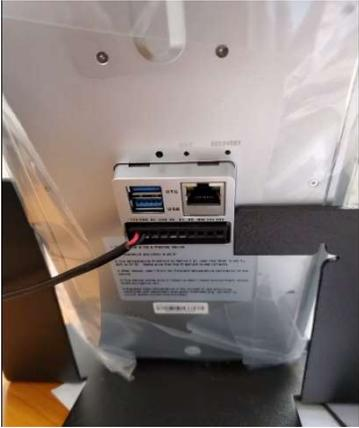
Connect the 10-position phoenix connector to the back of the PDI-TK8 unit (**Note:** the red power and black ground wires are on the left side of the unit as you're looking at the back of the unit). Next, plug the unit into the wall receptacle for power.
